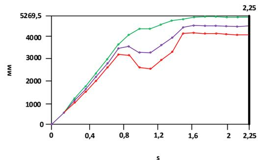
Figure 4: Graph of the movement of rock from the bunker to the conveyor belt.
